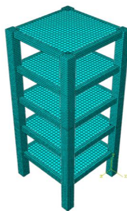
Gambar 3.10 Model 3D Portal 5 Lantai (Abaqus-Mesh)
