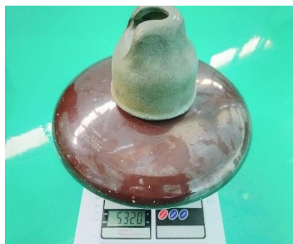
Gambar 3. 24 Massa Isolator Porselen Jenis Piring Keadaan Kering
