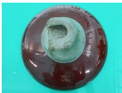
Gambar 3. 3 Isolator Gantung Jenis Ball and Socket
