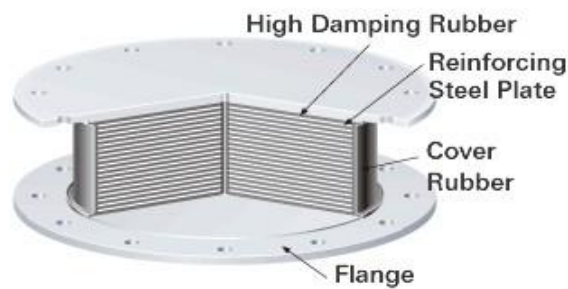
Gambar 2.3 High Damping Rubber Bearing
