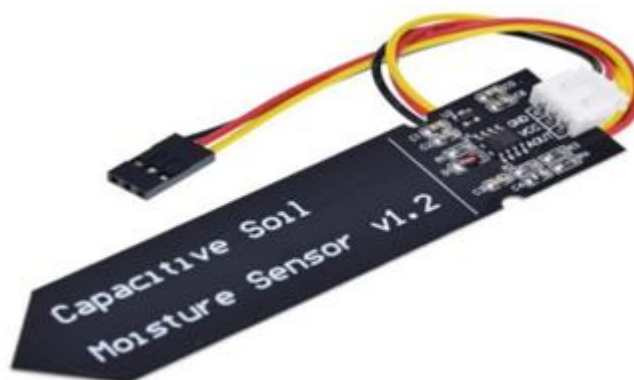
Gambar 2.3 Capacitive Soil Moisture Sensor v1.2
