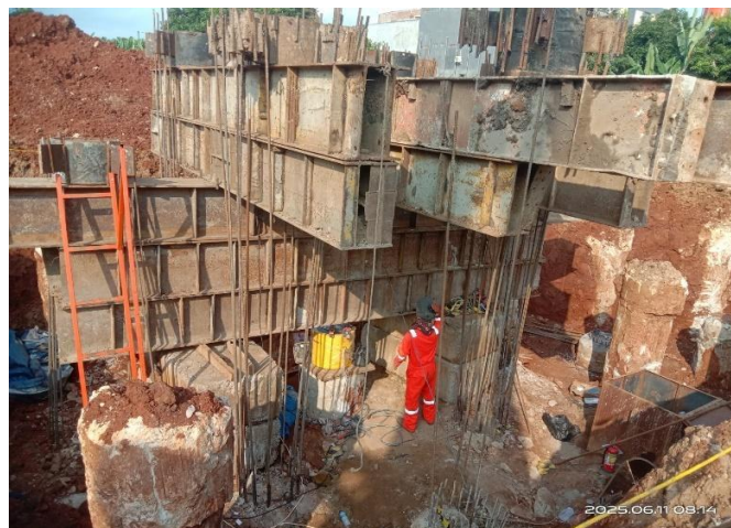
Gambar 2.7 Pelaksanaan Axial Static Loading Test
