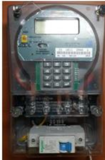
Gambar 2. 7 kWh Meter Digital Prabayar Sumber: (Fahraini Bacharuddin, 2017)
