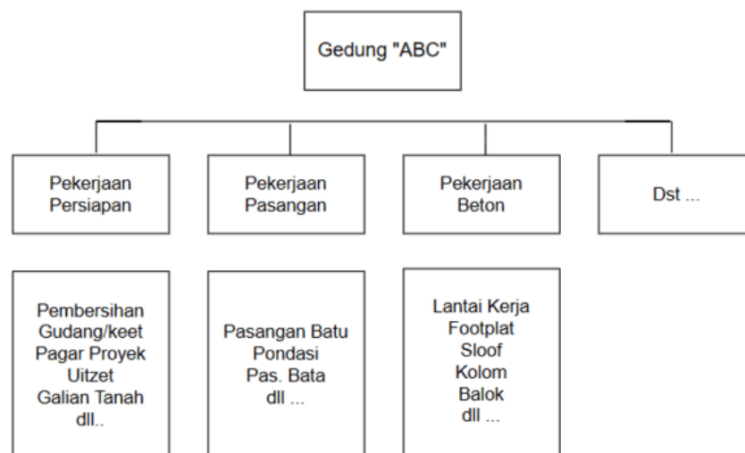
Gambar 2.6 Contoh Work Breakdown Structure (WBS)
