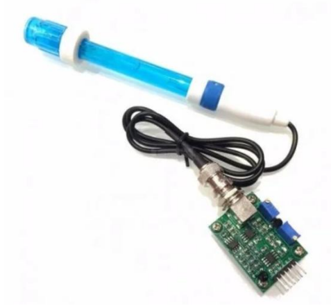
Gambar 2.7 Sensor pH-4502C with probe electrode Sumber: ssdielect.com
