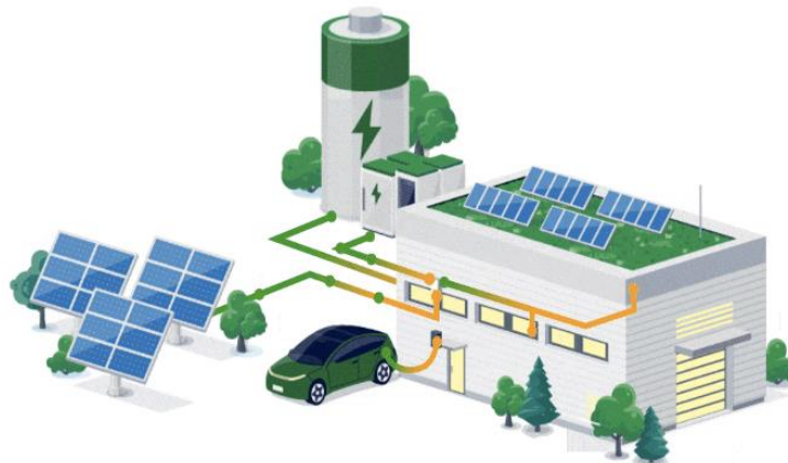
Gambar 2. 33 Sistem PLTS off grid (SUN Energi, 2023)
