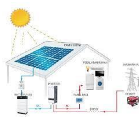
Gambar 2.7 Sistem PLTS Off-Grid (Naim & Wardoyo, 2017)
