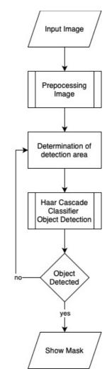
Fig. 4 Object Detection Flowchart with Haar
