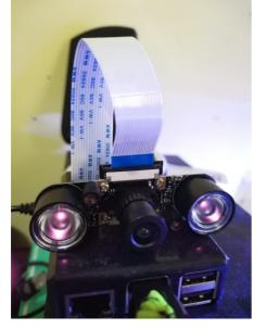
Fig. 3 Raspberrywith a camera module equipped with an IR sensor
