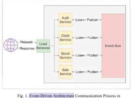
Fig. 1. Event-Driven Architecture Communication Process Microservice
