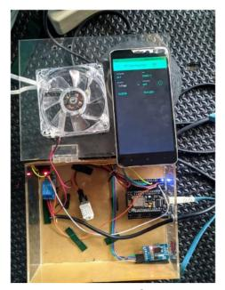
Fig. 10 The temperature is below  $30^{0}$ , and the fan does not turn on.
