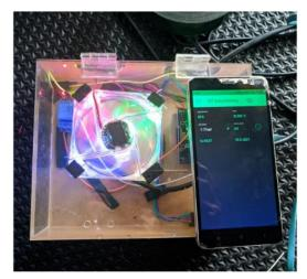
Fig. 11 The temperature is above 30°C, and the fan is on
