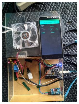
Fig. 10 The temperature is below  $30^{\circ}$ , and the fan does not turn on.
