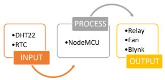
Fig. 2 Block Prototype Diagram
