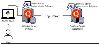
Fig. 1 NoSQL database document stored replication system architecture
