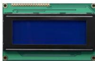
Gambar 2.16 LCD 20X4 (Ira Devi Gapy, 2017)
