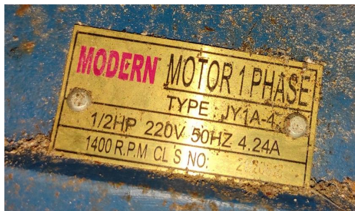
Gambar 3.4 Name Plate Motor
