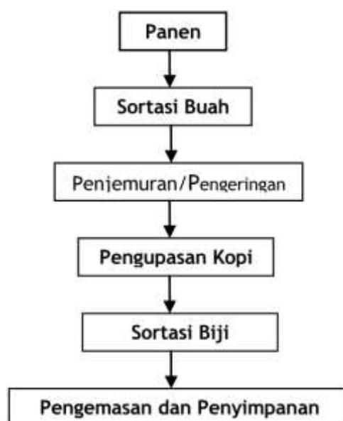
Gambar 7. Tahapan Pasca Panen Kopi Secara Kering (*Dry Process*).
