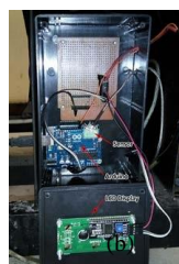
Figure 2. (a) Temperature control system circuit of the coconut sugar cooking system and (b) photograph of control system circuit.
