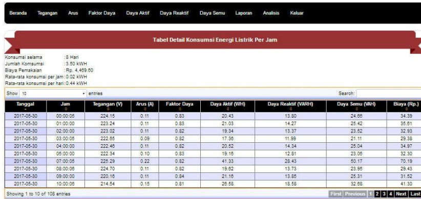
Figure 15. Power consumption in daily report dashboard.
