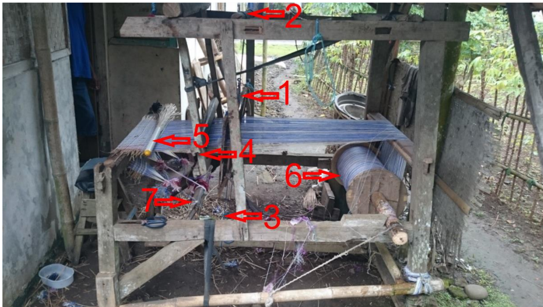
Gambar 2.16. Mesin Anyaman Mendong Tradisional Tustel (Hiron et al. , 2019)
