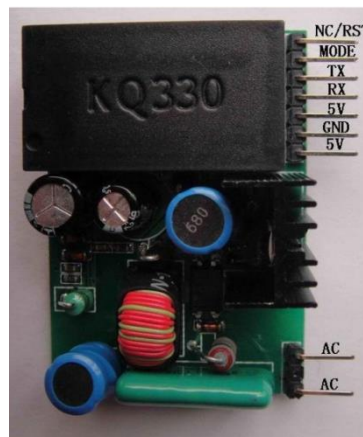
Gambar 3.5 Modul Power Line Carrier (PLC) KQ330
