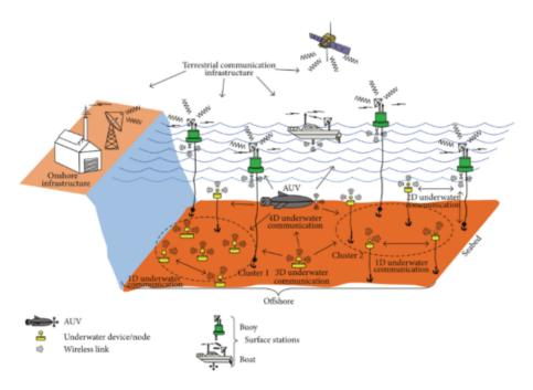
Fig. 2. Underwater sensor network architecture [11].
