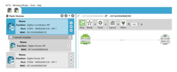
Fig. 8. Configuration of XCTU to determine the status of the remote module and local module.
