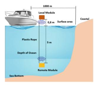
Fig. 4. Methodology of testing.
