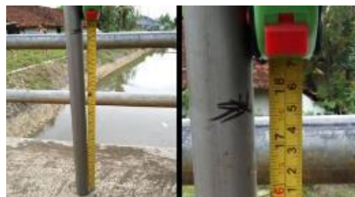
Figure 19. Validation of measurement result by measuring pole.
