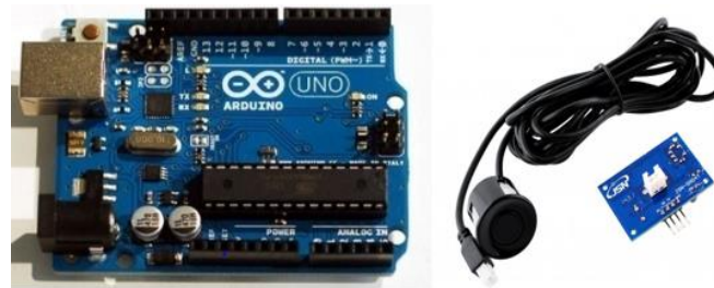
Figure 1. Arduino-Uno circuit board and JSN-SR04T sensor [6].
