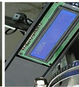
Figure 16. Water level testing at 100 cm.
