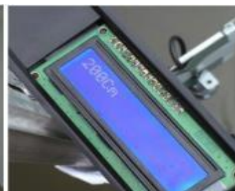
Figure 18. Water level testing at 200 cm.
