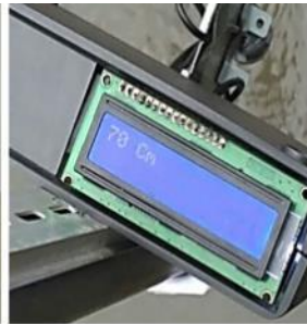
Figure 15. Water level testing at 70cm.
