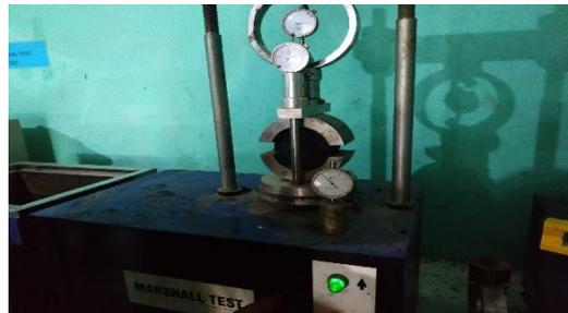
Gambar 1-4 Alat Uji *Marshall*
