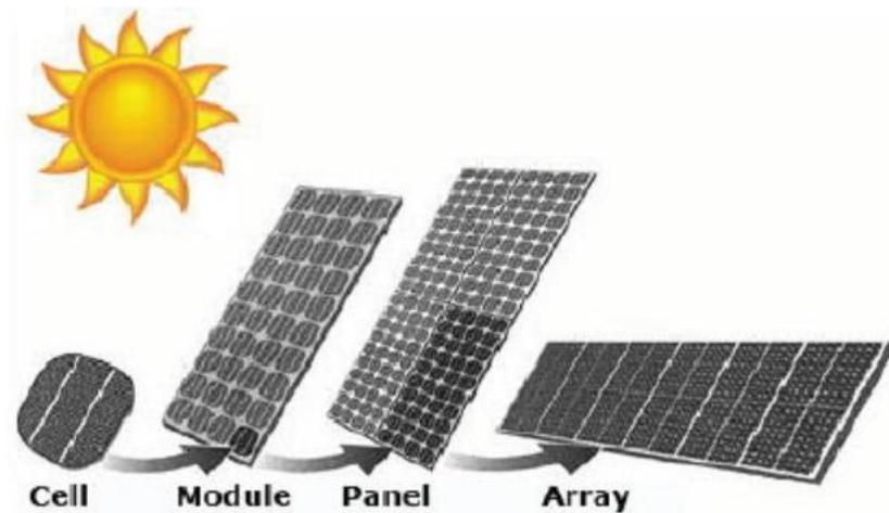
Gambar 2. 15 Cell, Modul, Panel, Array Surya (Pasangpanelsurya, 2022)
