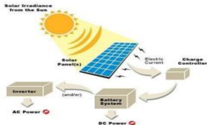
Gambar 2. 5 Sistem Kerja PLTS (Nugroho, Khwee and Yandri, 2022)
