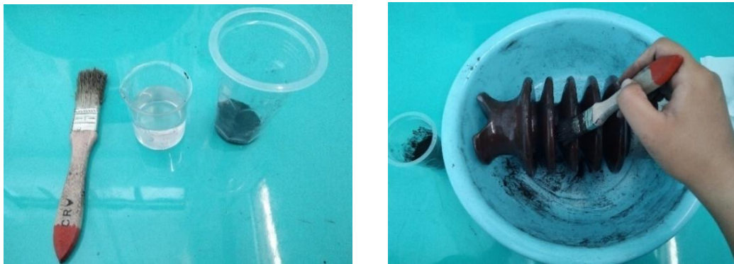
Gambar 3.3 Proses Pengotoran Isolator
