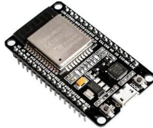
Gambar 2.2 Modul ESP32
