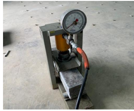
Hydraulic Concrete Beam Testing Machine
