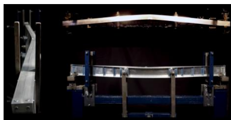
Gambar 2.23 Pola Kegagalan Lateral Torsional Buckling (LTB) (Sumber:
