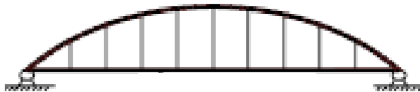
Gambar 2.3 Tipe Through True Arch (Sumber: Kementerian PUPR, 2021)
