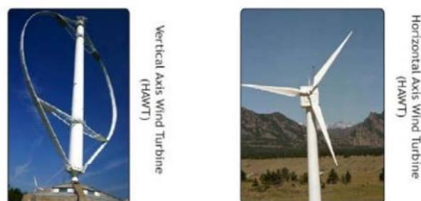
Gambar 2.1 Turbin Angin Vertikal dan Turbin Angin Horizontal (Hau,E et al.,
