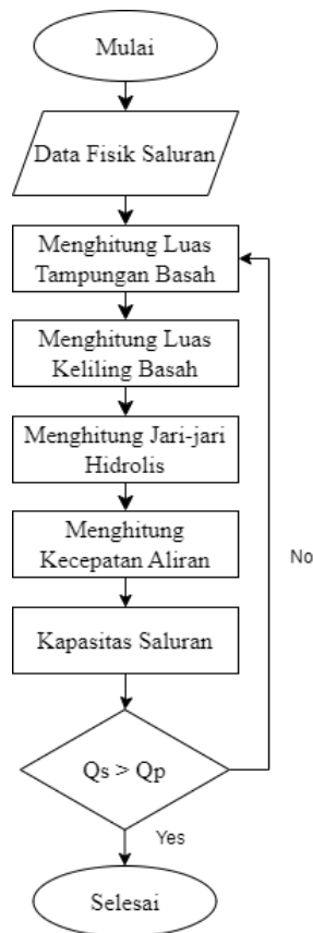
Gambar 3. 5 Flowchart Analisis Hidraulika
