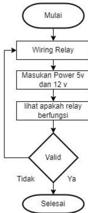
gambar 3.7 Flowchart pengujian relay
