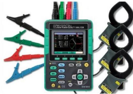
Gambar 3. 2 Power Quality Analyzer
