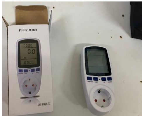
Gambar 3.5 Alat Ukur Power Meter
