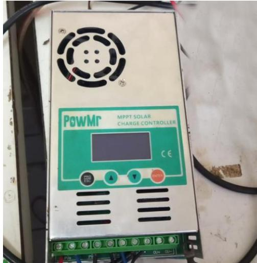
Gambar 2. 19 MPPT (*Maximum Power Tracking*)
